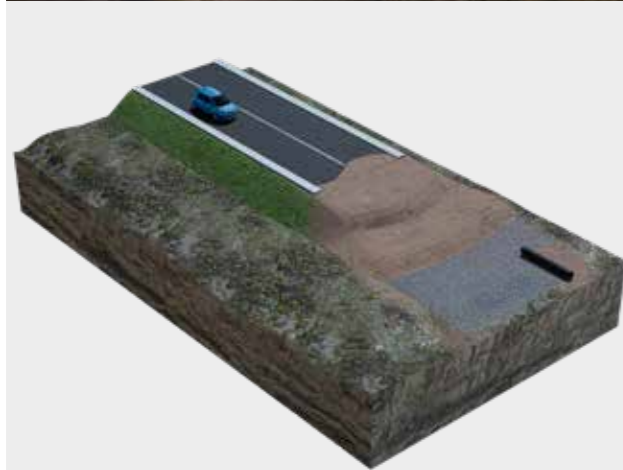
Embankment over soft soil
