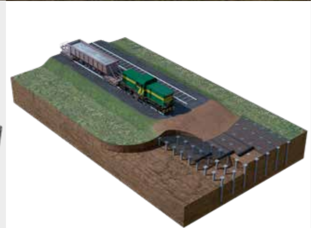
Embankment over rigid inclusions
